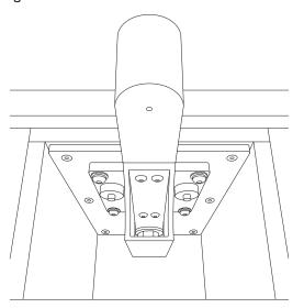
Place the countertop top-side down on the floor and align mounting holes of the unit plate to the threaded inserts in the bottom of the countertop. Attach using the 1/4"-20 x 1" long screws and lock washers in the hardware kit.
