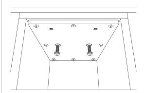
Slide the leveling assembly onto the bolts that are pre-installed in the mount plate. Then add the 2 3/8"-16 bolts and accompanying washers to the remaining open holes in the leveling plate. Then tighten all 4 bolts.
