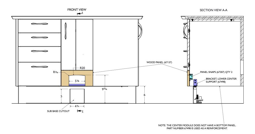
SOLUTION 1: DCI 12 O'CLOCK CABINET AND COMPONENTS - LOWER MOUNT INSTALLED
