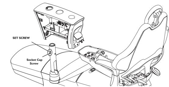
2 Secure the PMU against the post by tightening 2 set screws as shown below. Re-install the tension adjustment screw and the rotation stop screw. To avoid damage to the post bushing, Do Not Tighten the tension adjustment screw until after the S-Pole has been installed.
