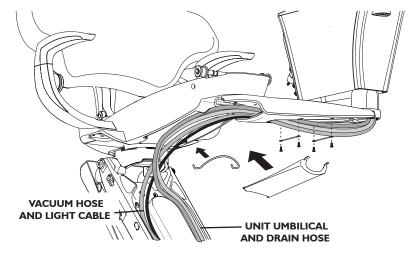
6 Reattach the PMU mount wires with the fours screws as shown. Reattach the wire hanger by pointing the hooks upward, pushing them into the holes nearest the swivel of the chair, and then rotating the hanger forward.
