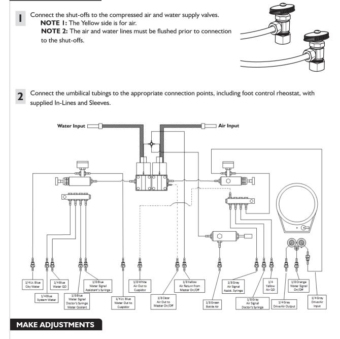
See the ADJUSTMENTS section near the end of the **Instructions For Use** Manual for the **Series 5 Delivery System** to complete the installation. Be sure to check and make any needed adjustments to items in that section.
