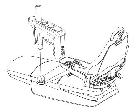
Keep the PMU parallel to the chair and secure the PMU in the 2" hub by tightening the eight set screws located in the hub. Use a post level or two magnetic levels to keep the PMU Post level while tightening the set screws.
